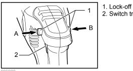
1. Lock-off button 2. Switch trigger
